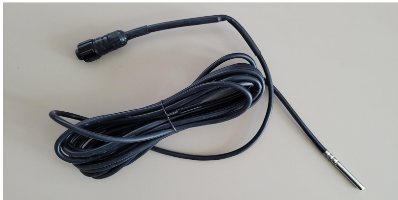
Figure 4. Soil temperature sensor
