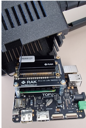
Figure 2.3 Photo of the intern composition of the SG-Box device
