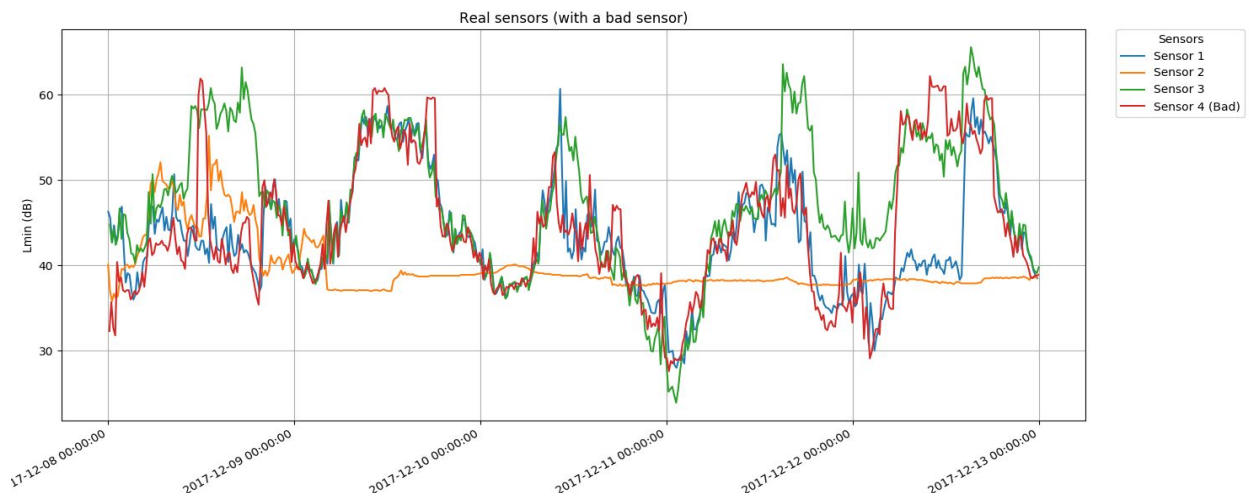
Figure C.4 : Datasets representing real sensors with a bad sensor
